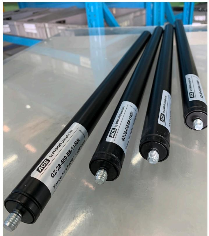
*The ACE Controls' GS-28-450 pull-type gas spring provided a 270-pound traction force and low progression rate to hold the mobile X-ray device's beam arm in the final position and support raising and lowering motion.*
